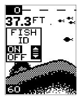
The Fish ID feature can't be used when the X-45 is in the manual mode. If you turn the automatic feature off, the Fish ID feature will automatically be turned off, also.
